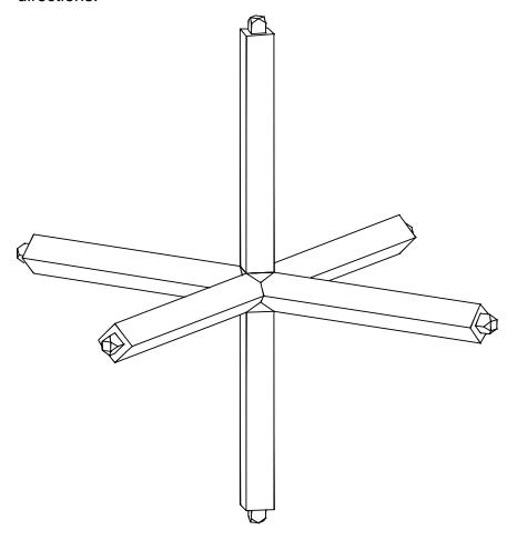
4. By inserting into slots, the construction assemblies may be achieved in orthogonal directions
