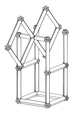
6. To enhance the stability or rigidity of the construction, the additional diagonal poles are inserted on the inner or outer side.
