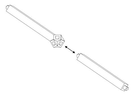
3. Thorn of pole element may be inserted int the puzzle head in five orthogonal directions.
