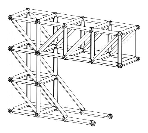
7. If triangle fillings are inserted into inner diagonal element, closed surfaces may be gained.
